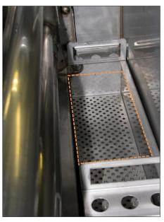
3. Open the cover using the two thumb screw on each side of the unit while the humidifier is being drained. There are two covers on the humidifier. A painted cover that is on the top and a stainless steel cover beneath it.
